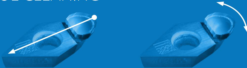
When cleaning the tool (on or off the machine) use **isopropyl alcohol or acetone** and a lint free cloth or a Q-tip. Always wipe along the front of clearance angle along the cutting edge. Paint brushes and un-filtered compressed air can hold particles that can cause damage, so are not recommended. Never drag anything from the top of the diamond over the cutting edge, as this may cause a chip-out.
